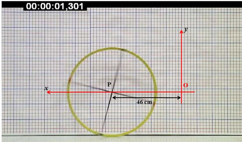
Figure 1: Distances must be measured from the origin  $O$  to the center of the ring,  $P$ , in this frame 23 red squares = 46 cm. The time is 1,301 s.
