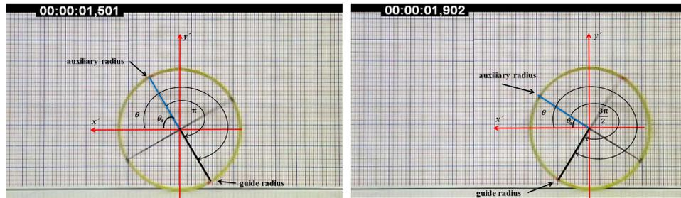
Figure 4: Corrections for measurements in the first quadrant when the guide-ray is in the third quadrant (left) and fourth quadrant (right).
