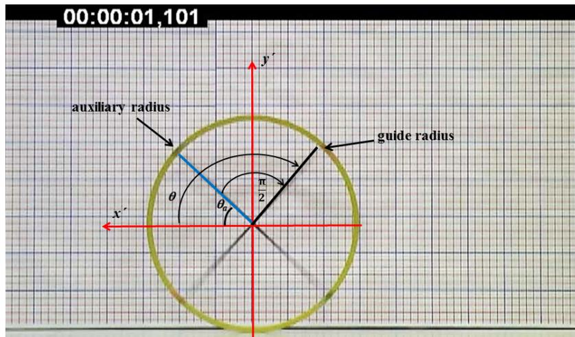
Figure 2: The angular position of the guide radius in the second quadrant can be obtained from the angular position of the auxiliary radius by adding  $\frac{\pi}{2}$  to the value measured in the first quadrant.
