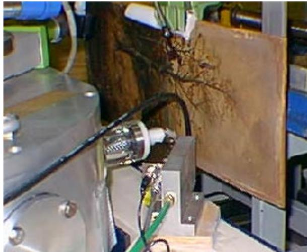
**Figure 2. View of the multi-use chamber with the new external beam setup installed and the X-Ray detector (XR-100CR) and the painting.**
