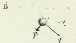
(c) If \vec{v} is not \perp to \vec{B} , there is a smaller force, proportional to v_{\perp} instead of v .
