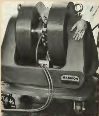
A modern electromagnet used in research when strong uniform fields are required.
