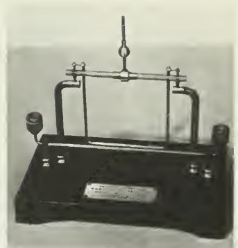
Replica of Ampère's current balance. The essential part is a fixed horizontal wire (foreground), and just behind it, hanging from a hinged support, a shorter segment of wire. Current is produced in both wires, and the force between them is measured.
