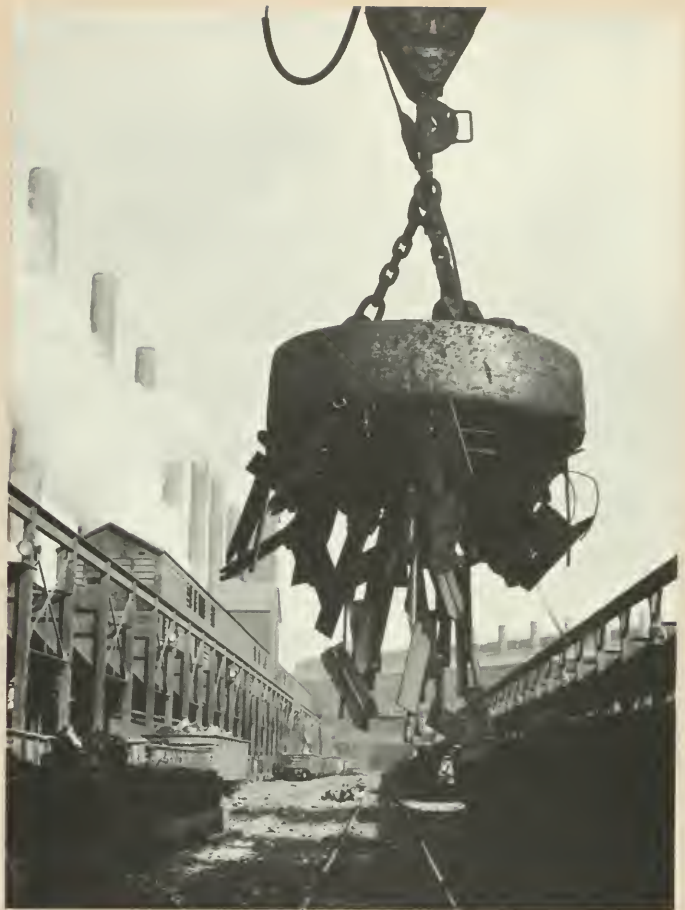
The first electromagnet, invented by William Sturgeon in England in 1824, could lift a weight of nine pounds. In 1832, Joseph Henry constructed an electromagnet at Princeton which could hold up a weight of 3,600 pounds. Modern electromagnets (see above) which can typically lift 50,000 pounds of iron are widely used in industry, for example, to sort or load scrap metal.
