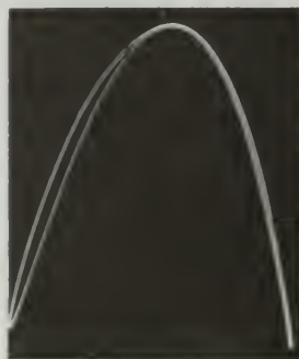
Fig. 17 Frequency 2 to 1 with 90^\circ phase difference.
