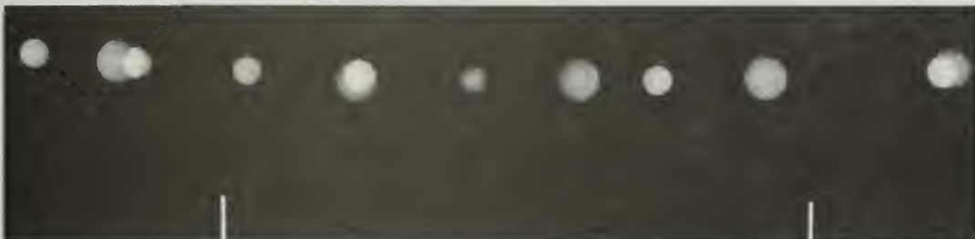
Stroboscopic photograph of the entire Event 4. 10 flashes/sec. Both balls cross the field of view in the same direction (from left to right) as time goes by. It is not easy to analyze this picture. Handbook Fig. 3-14 shows how this difficulty was resolved.
