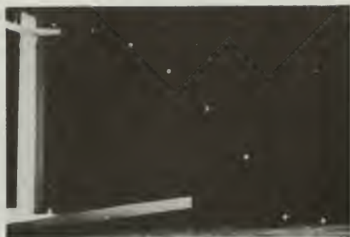
Fig. 5 Xenon strobe photograph of trajectory of steel ball. Strobe rate about 20/sec. Aperture setting of EV 16 on models 800 and 150; EV 7 on model 95. Film selector to 3000 on model 320.
