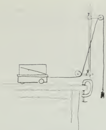
Fig. 9 Arrangement to demonstrate uniform acceleration.
