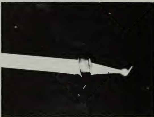
14-3. Convergence of light by a cylindrical lens like the one shown in Fig. 14-1. Note that the light is brought to a focus along a line.
