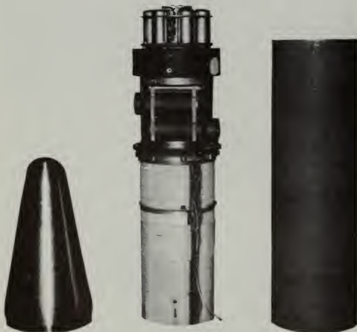
HEAD OF EXPLORER IV includes nose cone (left), instrument "payload" (center) and protective shell (right). Payload includes four detectors, two radio transmitters, batteries and associated electronic circuitry. The outer shell is approximately six inches in diameter.
