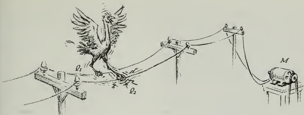
FIG. 40.13. The voltage drop between Q_1 and Q_2 might be great enough to kill the bird.
