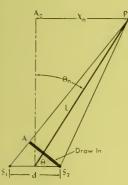
Now draw a line from  $S_2$  to A such that  $PS_2 = PA$  (see diagram). Then  $PS_1 - PS_2 = AS_1$ . Assume that P is far enough so that  $PS_1$  and  $PS_2$  are nearly parallel and that angle  $S_1AS_2$  is a right angle. Then  $Sin \theta = AS_1/d$  (Identify angle  $AS_2S_1$  as  $\theta$ ).
