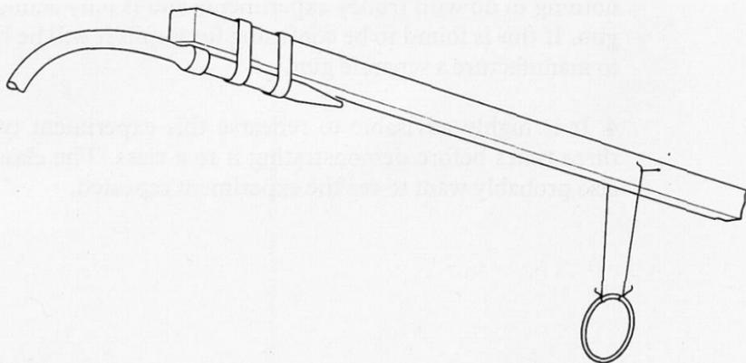
At equal distances from the end of the jet, pairs of panel pins are hammered into the pole or beam as shown.
