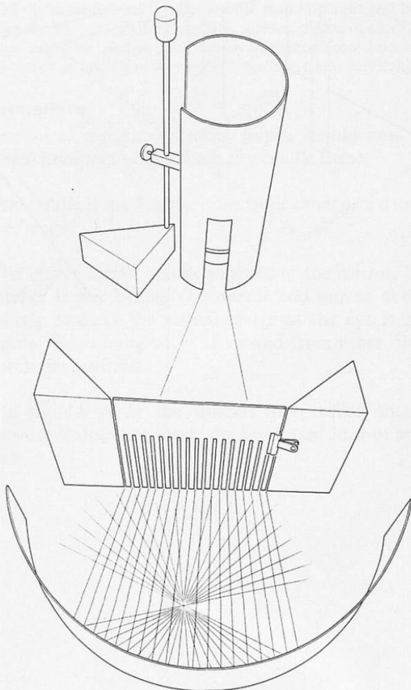
This illustration shows the arrangement of apparatus and the 'ideal' behaviour of rays that we would like to find. Pupils will be surprised and pleased when they see the real behaviour. Then the continuation of the experiment, with a narrow fan of rays, will show when a proper image is formed.
