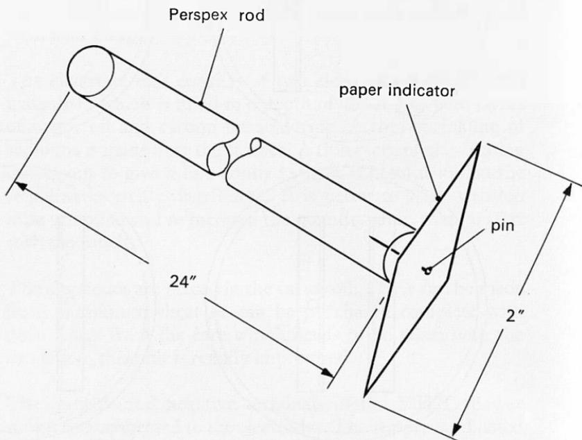
class. The E.H.T. power supply is switched on and the indicator sets along the field lines.
