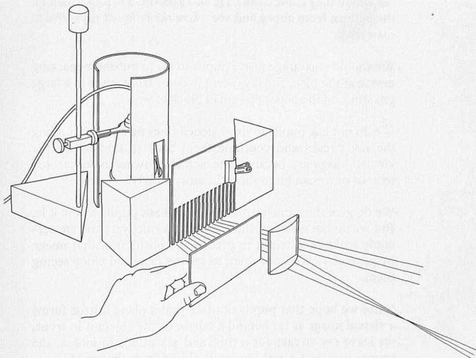
*o. Plane mirror receiving a fan of rays from an object*
