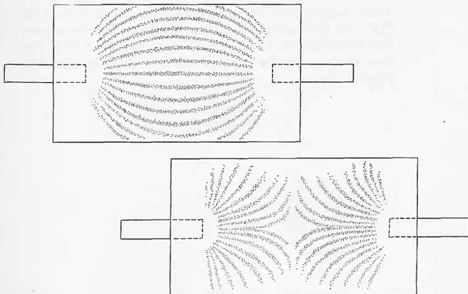
4. Instead of the ticonal magnets, use two magnadur magnets. Again investigate the field using both iron filings sprinkled on card and the exploring compass. The magnadur magnets can be put on the bench as shown, or attached to the iron yoke.
