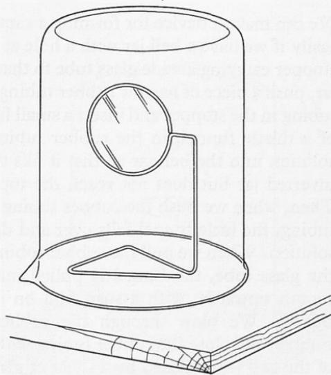
The Stergene solution is put into the beaker and a film formed on the frame. This film is then used as a mirror to reflect light from the window to the class. As the film drains interference bands are seen.
