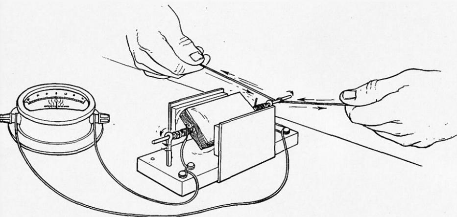
87b *Optional class experiment***Electromagnetic induction: motor as a dynamo
