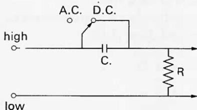
In the A.C. position there is a capacitor in series with the input and this will separate the a.c. component from a wave form such as :
