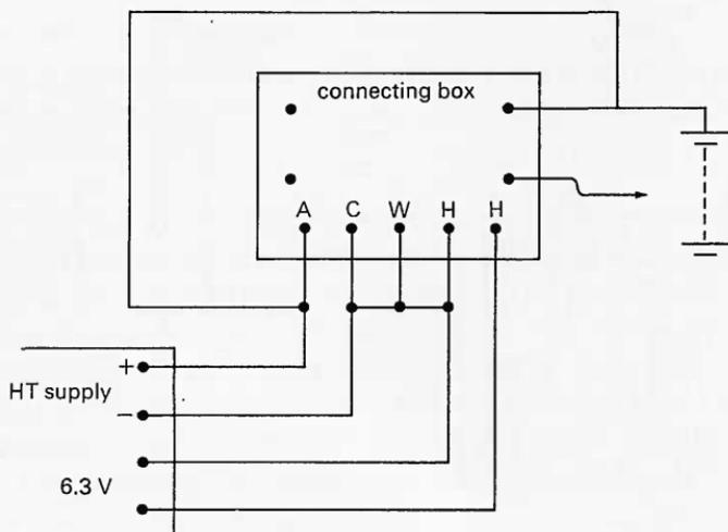
Before switching on check that the power supply potentiometers are set so that the anode potential will be zero. Turn the tube so that the electron gun points vertically upwards.
