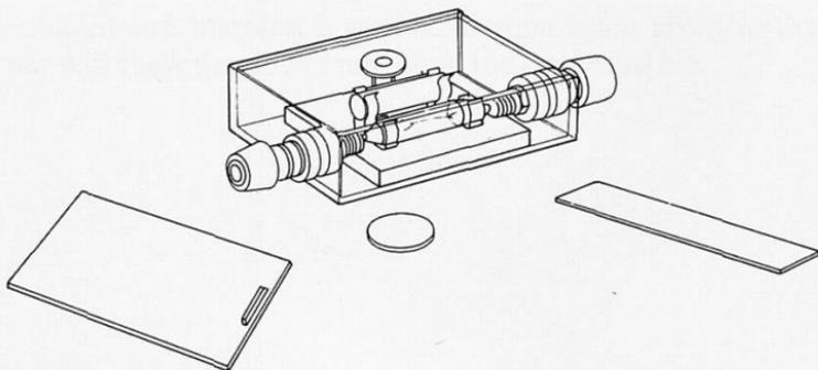
Light the end of a piece of cord (sash cord, clothes line, or a drinking straw are suitable) and allow to burn for a few seconds. Blow out the flame and fill the dropper with smoke from the smouldering cord. Inject the smoke slowly from the dropper into the glass cell. When it is full, seal with the cover slip provided.
