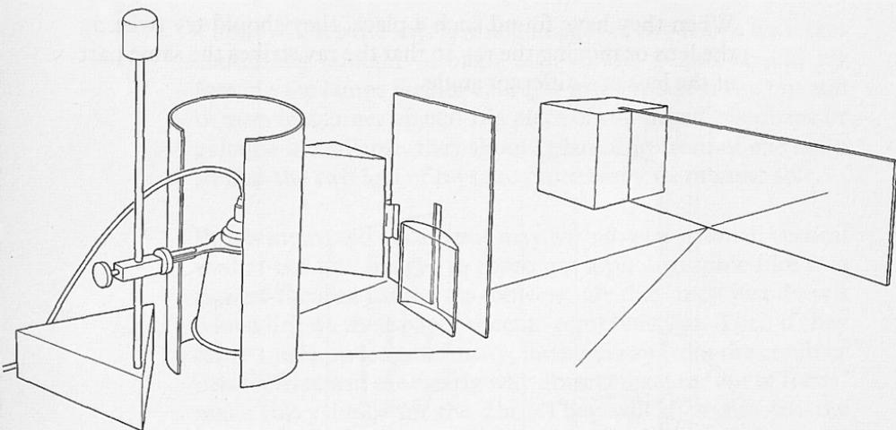
k. *Optical centre : undeviated rays, using +7D lens*
