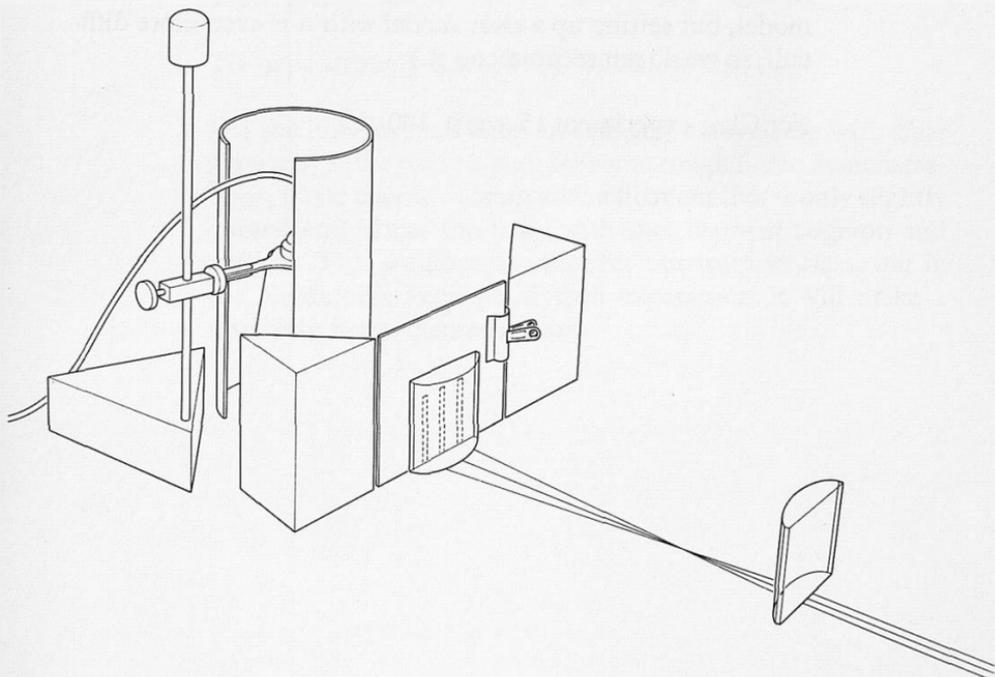
The objective lens is a strong positive lens, +10D. The screen with three slits is placed close to it and the lamp again serves as an object. The curved face of the lens should be away from the lamp.
