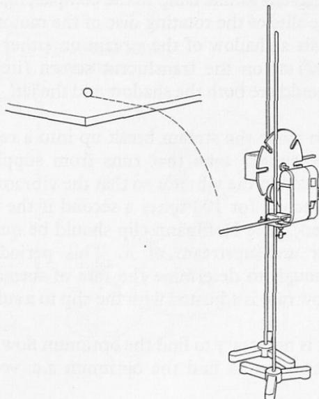
67 *Demonstration***Pulsed water drop experiment****Apparatus**
