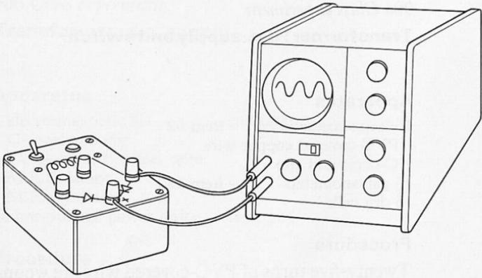
90a *Class experiment***Transformer: d.c. supply and switch****Apparatus**
