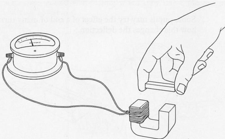
88d *Class experiment***Electromagnetic induction using an electromagnet****Apparatus**
