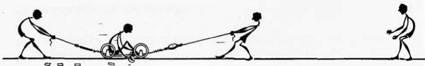
This is repeated with other backward drags and discussion of the results should enable a guess to be made at the force of friction's concealed backward pull. The result can be tested by pulling the trolley with exactly this amount to see if it is just the force to maintain constant velocity.
