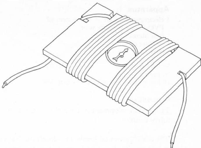
If this device is placed on the bench so that the needle is parallel to the winding, quite small currents will cause readily observable deflections to E or W according to the direction of the current. If connection is made to the power supply through a 100-ohm carbon resistor, the small current (about 10 mA) gives an observable deflection. The pupils should also try with a 10-ohm carbon resistor. Direct connection with no resistor sets the needle spinning.
