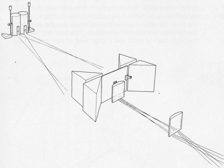
r. *Optional. Use of a field lens in a telescope (using  $+17D$ ,  $+7D$ , and  $+7D$  or  $+10D$  lenses)*
