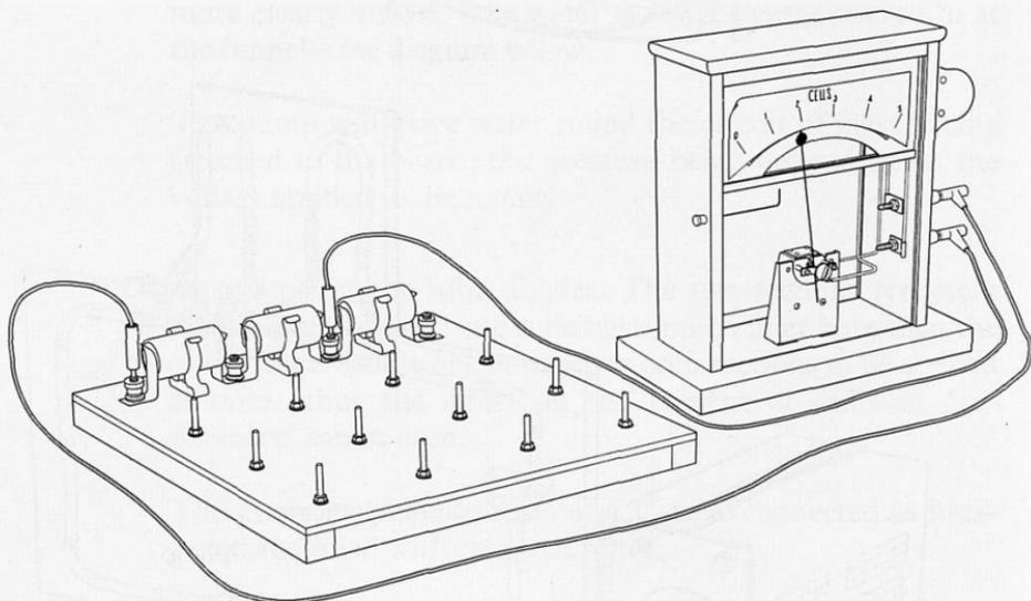
The board is then fitted with three lampholders in series. The demonstration meter is put across the three lampholders. First *one* cell is connected across the three lamps and the demonstration meter reads approximately '1 cell'. Then two cells are connected across the three lamps and the demonstration meter reads approximately '2 cells'. Then three cells across the three lamps.
