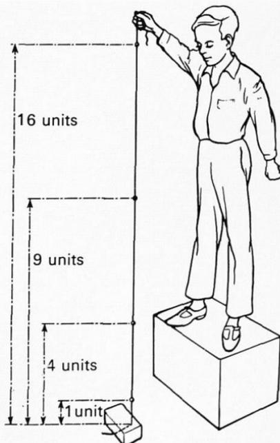
A string is anchored at the end by a brick resting on the floor. The pupil attaches loads to it at suitable distances. He holds the other end of the string high above the floor, keeping it taut, and lets it go.
