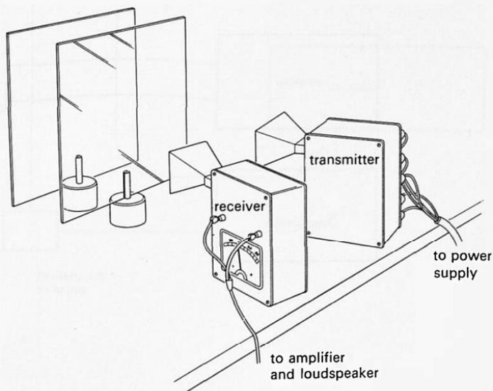
39c *Optional demonstration***Interference using sound waves****Apparatus**
