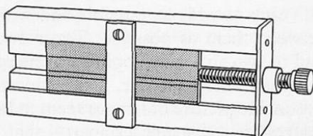
The slits are made by coating one side of a microscope slide with Aquadag. The slide is inserted in the holder and a slit ruled on the Aquadag with a blunt needle or pin held up against the brass cross-piece. The edge of a small screw-driver can be used. Even a fine ball-pointed pen works well in practised hands.
