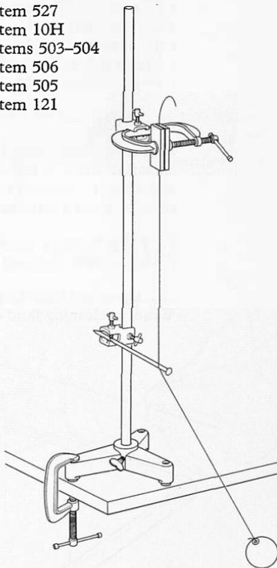
For success in this experiment it is essential to have a massive and very rigid support for the pendulum and for the 'pin'. Otherwise energy is lost at the support.
