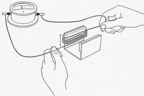
*88c Class experiment***Electromagnetic induction : magnet and coil on iron core****Apparatus**
