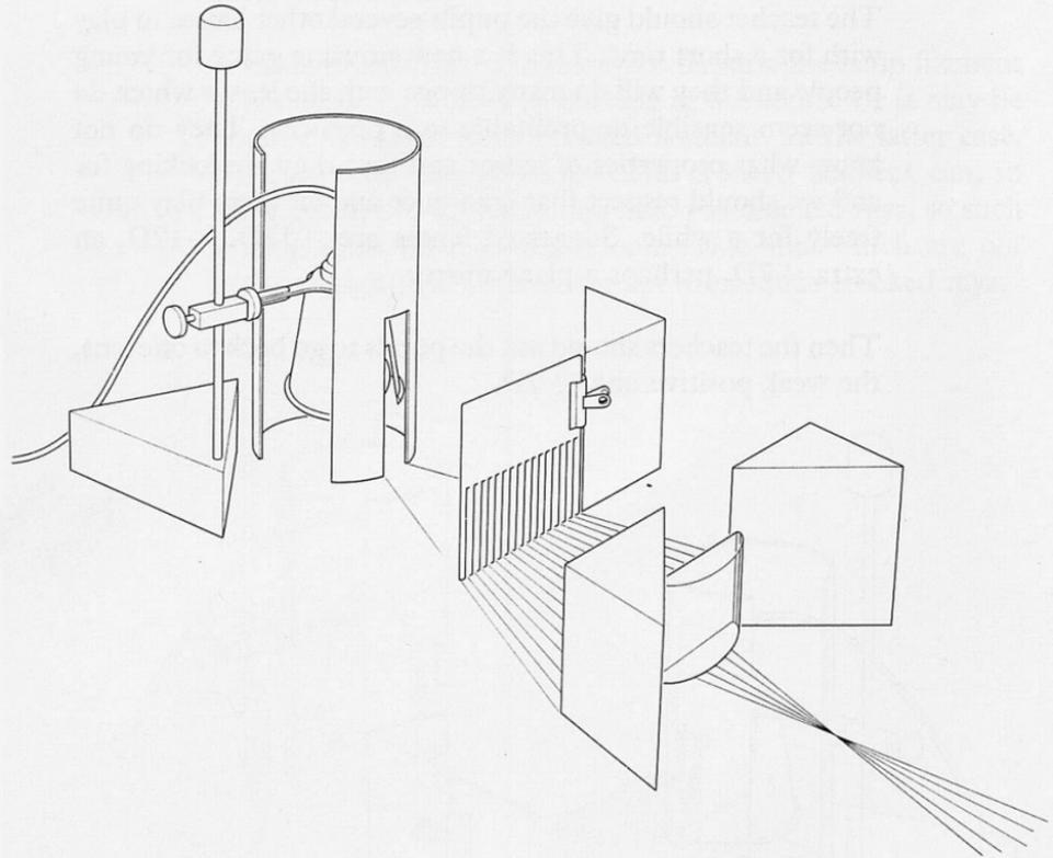
d. *Fan of rays and two lenses (both  $+7D$ )*
