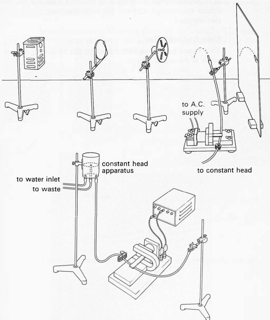
The above will have shown that the vertical motion is accelerated. To demonstrate that the horizontal motion has constant velocity, impose a rectangular grid or project the shadow on a screen ruled with squares.
