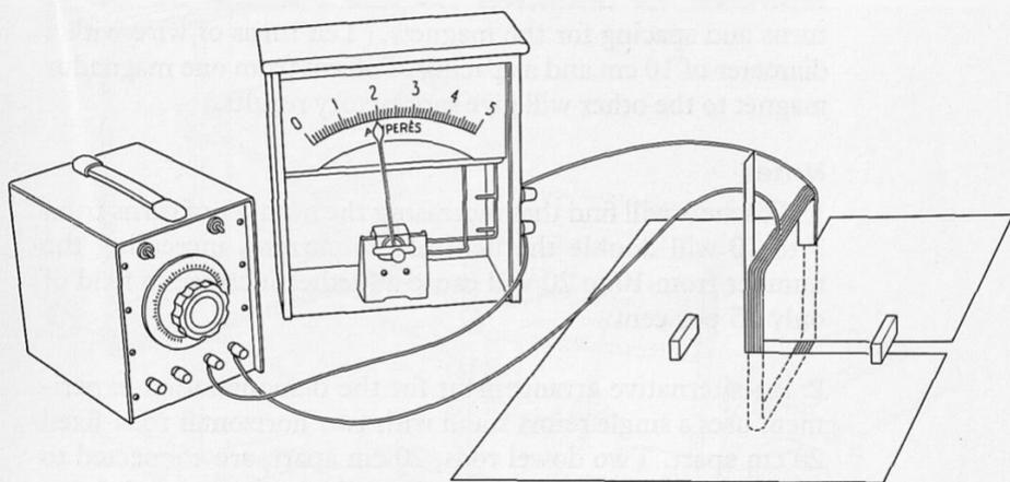
Put a piece of paper with a slit in it on the hardboard. Place on it two magnadur magnets 15 cm apart with unlike poles facing. Sprinkle iron filings on the paper. Switch on and turn up the voltage until 3 amps flow. Tap the paper sharply with a pencil.
