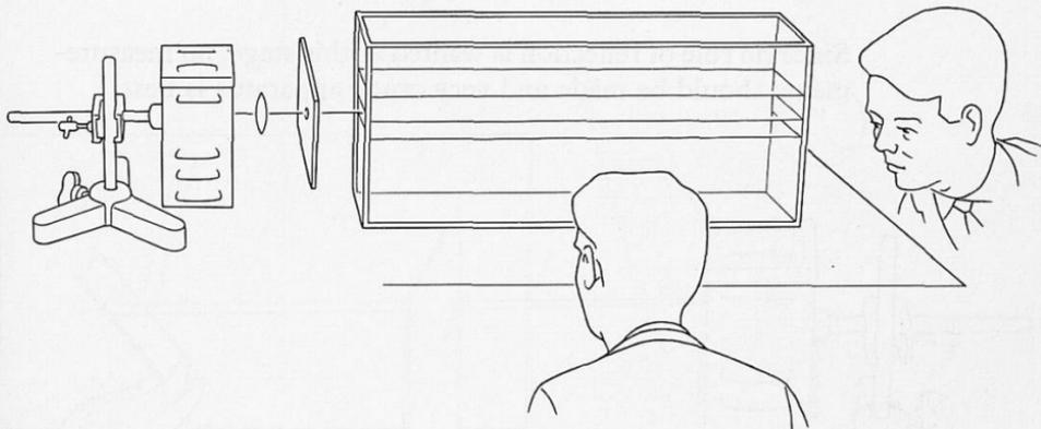
6e *Demonstration***Ray of light being reflected****Apparatus**
