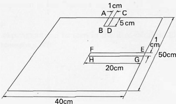
Connect the ends to the d.c. terminals of the L.T. variable voltage supply via the meter reading to 5 amp.
