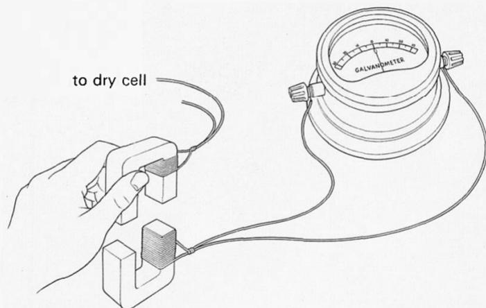
*88e Class experiment***Electromagnetic induction: switching an electromagnet****Apparatus**
