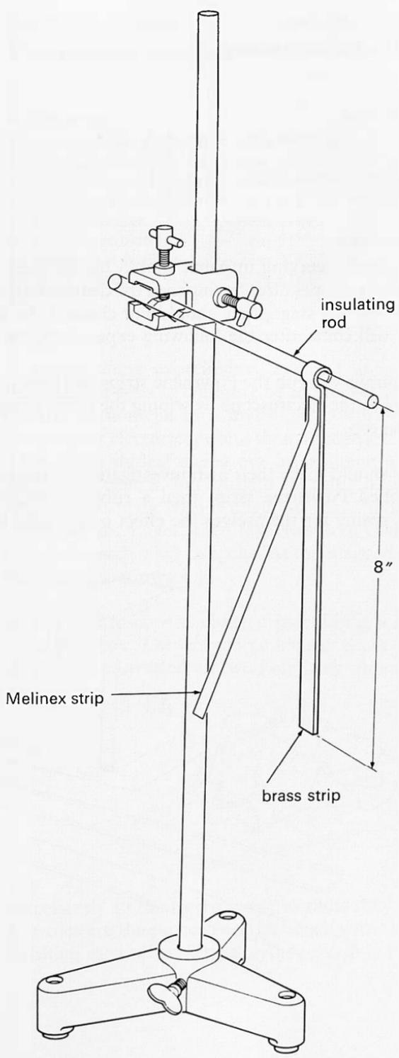
*99c Class experiment***Gold leaf electroscope****Apparatus**
