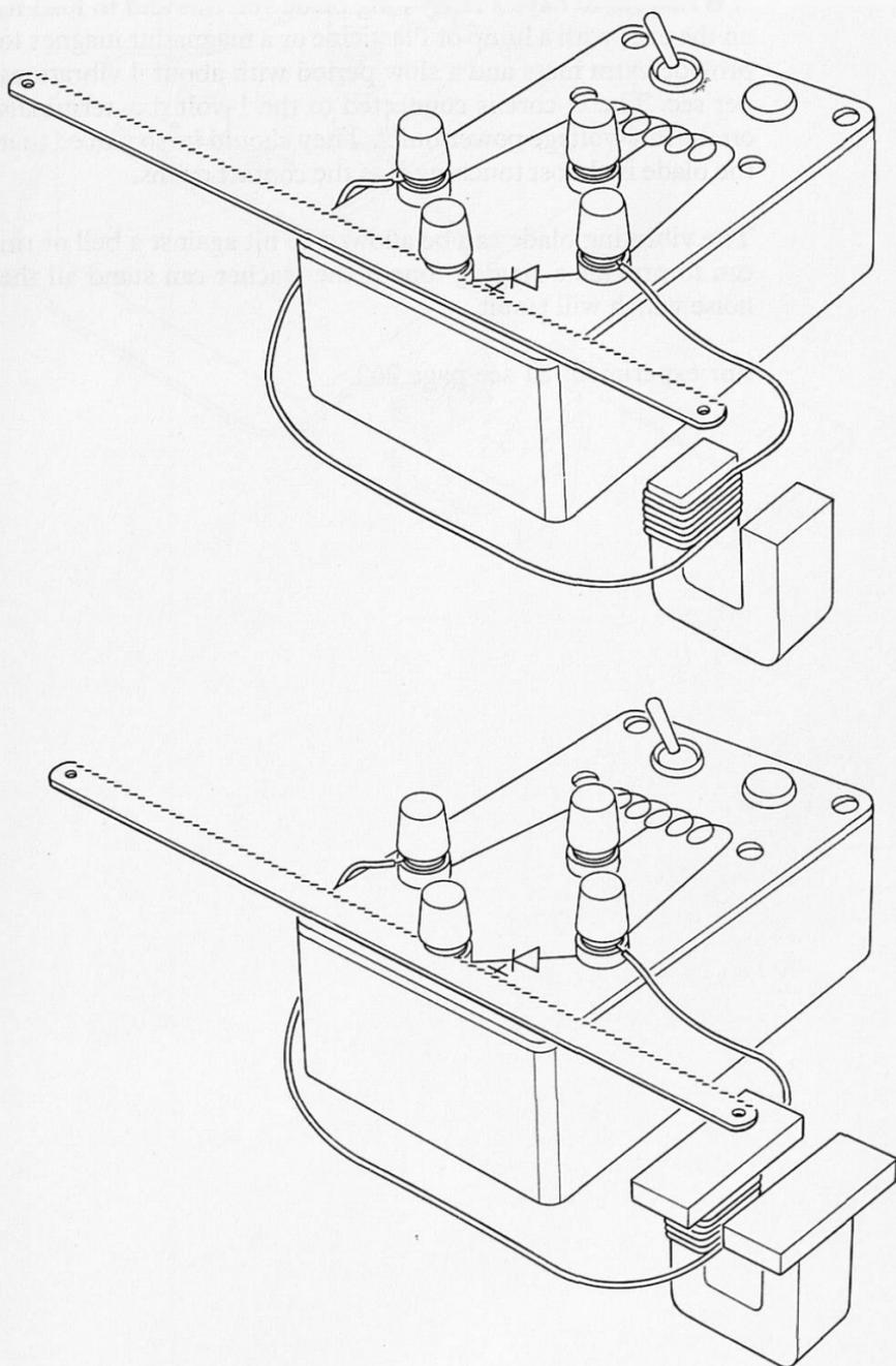
2. To make a contact breaker as in an electric bell, wires may be Sellotaped as shown opposite.
