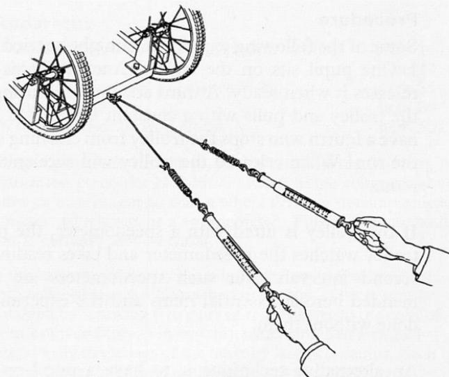
4. They are then repeated with three equal pulls of, say, 1 kg weight in parallel. It is not easy to apply the three forces in this way, but a little practice (and the avoidance of large boys) makes it possible.
