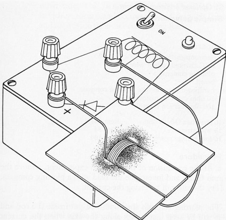
81 *Optional buffer experiment***Simple galvanometer****Apparatus**
