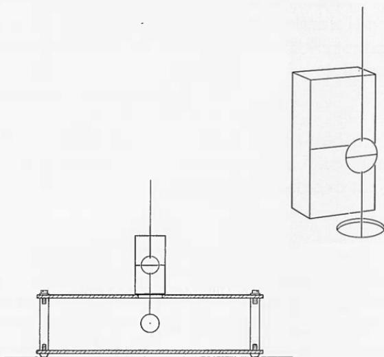
There are no measurements to be made in this demonstration: it is a qualitative experiment to demonstrate the principle of a force on a charged body between two parallel plates. In any case, there is a tendency for the charge to leak away along the suspension and quantitative experiments do not lead to very satisfactory results unless considerable trouble is taken and that is not justified at this stage of the course.
