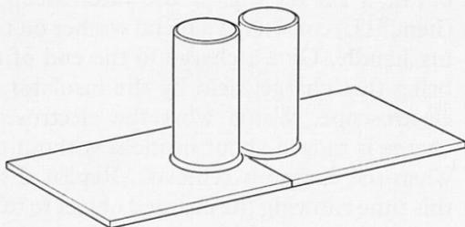
successively to the electroscope to show they are uncharged. The tiles are then placed on the bench with the two canisters touching each other. The Polythene strip is rubbed with the
