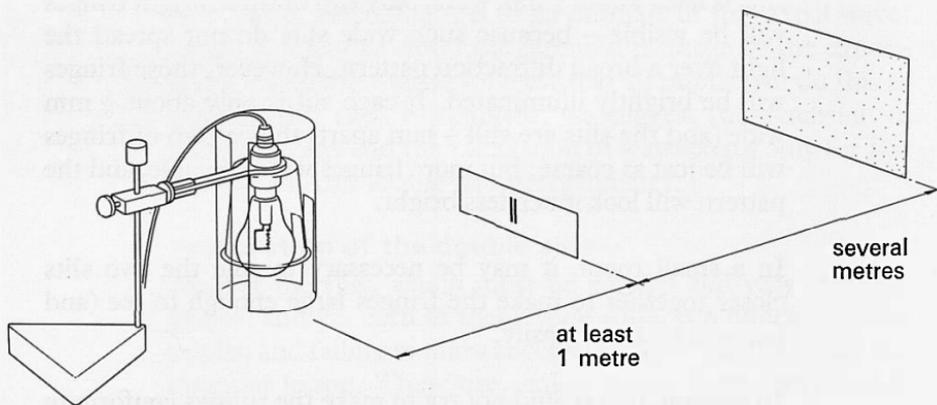
The teacher will find it necessary to help the pupils to orient the slits parallel to the filament of the lamp since this is an important adjustment for obtaining clear fringes.
