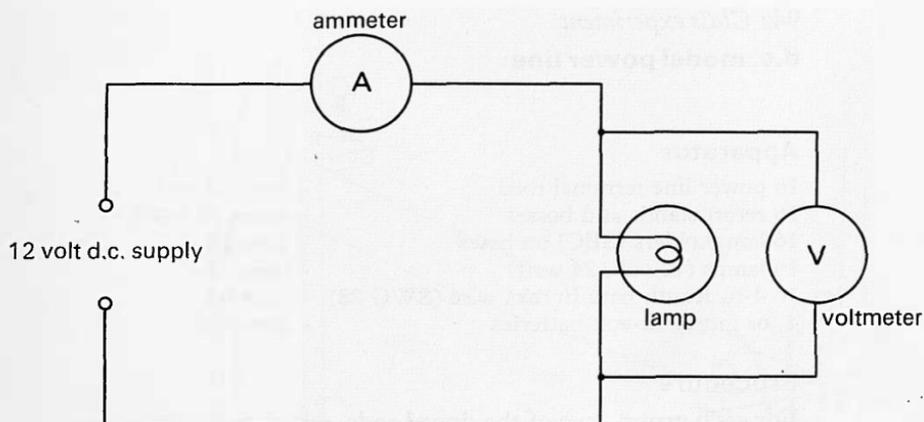
94a *Class experiment***d.c. model power line****Apparatus**
