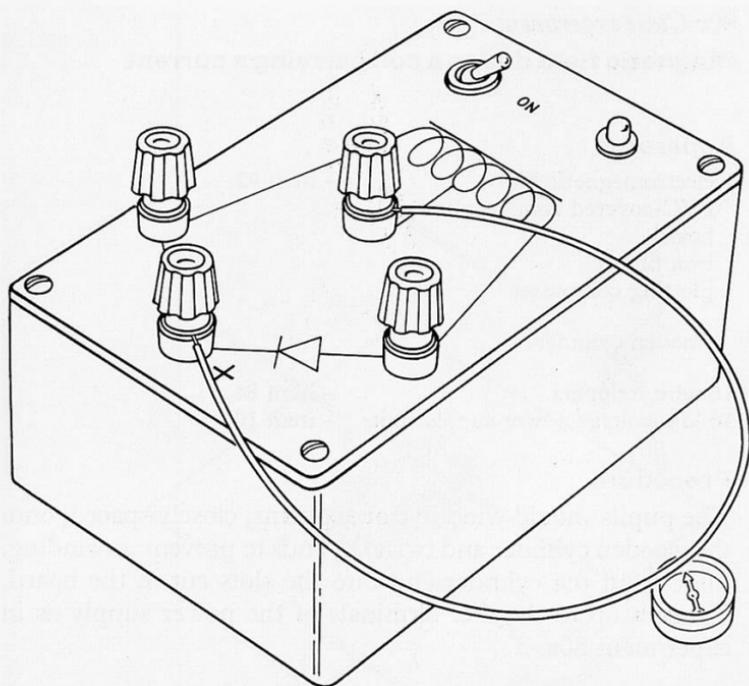
*80c Class experiment***Magnetic field due to a coil carrying a current****Apparatus**
