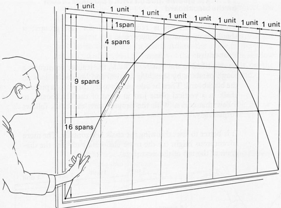
*68b Optional demonstration***Water jet following a parabola drawn on the black-board****Procedure**
