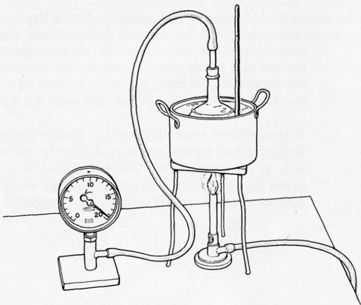
The flask should be tilted (or placed in a deep container) so that it is fully covered by water, right up to the top of the neck. That is not essential in this *qualitative* demonstration, but it should be done here to set a good example for the *quantitative* class experiment that follows soon, (77).
