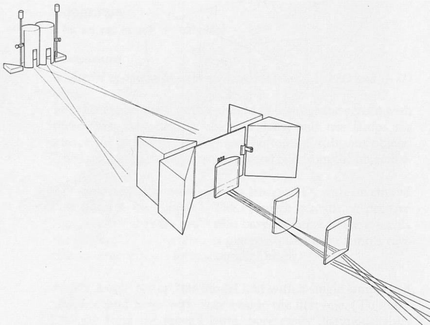
s. *Model of a microscope with ray streaks (using +10D, +17D lenses)*
