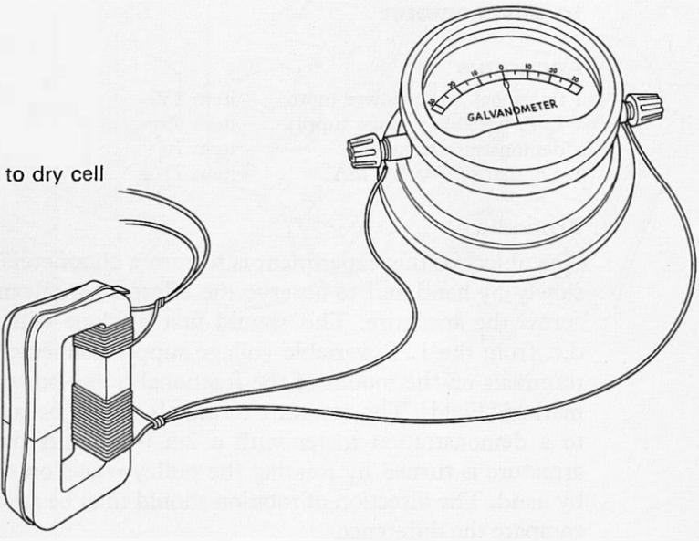
88f *Demonstration***Electromagnetic induction : FHP motor connected to galvanometer****Apparatus**
