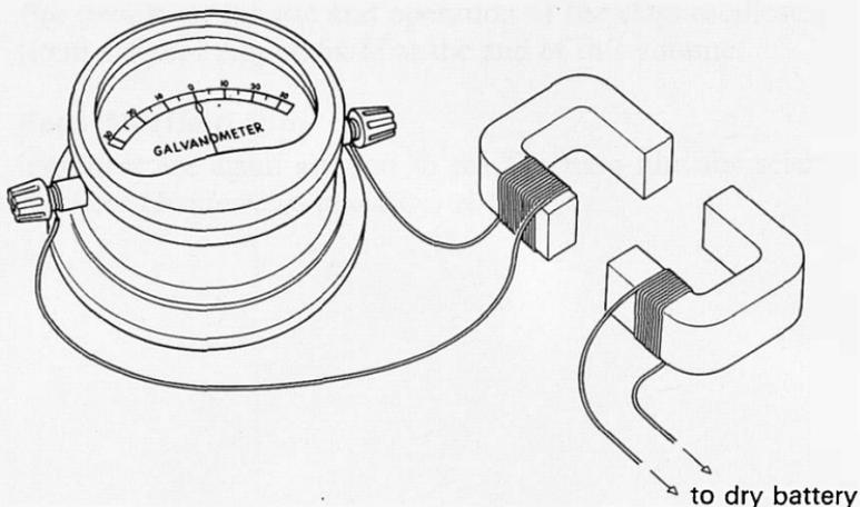
90b *Class experiment***Transformer: a.c. supply****Apparatus**
