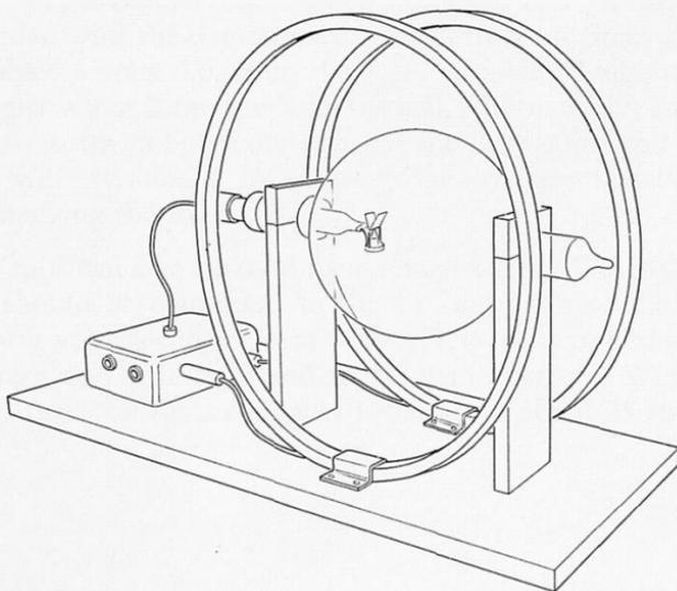
3. Should the beam appear very diffuse at all voltages between 150 and 250, apply up to +6 volts to the Wehnelt cylinder – this may sharpen the beam. Should the trouble continue, return the tube to the makers as it is not doing them justice.
