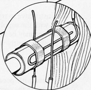
would suffice – but the loop enables contact with the brushes to be maintained over a greater part of a revolution with a consequent increase in power.
