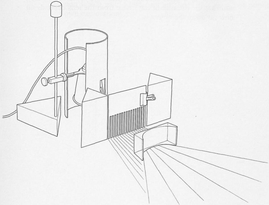
*g. Effect on image of changing object distance (using lens +7D, later with +17D)*
