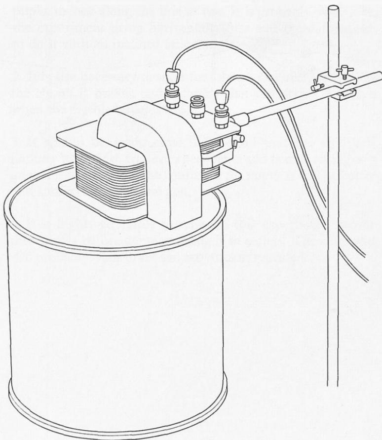
The trigger mechanism to release the 'monkey' is a strip of aluminium foil, across the end of the launching ramp. This strip is included in the circuit of the electromagnet holding up the tin. The position of the foil is such that the marble breaks it at the moment it leaves the ramp.
