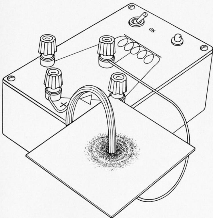
*80b Class experiment***Oersted's experiment****Apparatus**
