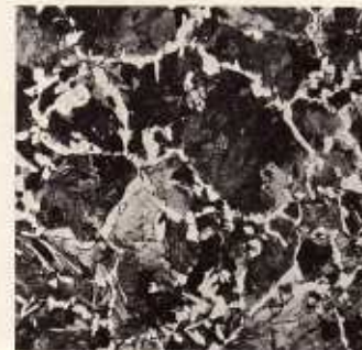
'Pearlite' structure of a carbon steel bottom . The iron and iron carbide are in very thin alternate layers (magnification \times 2000 ). National Physical Laboratory
