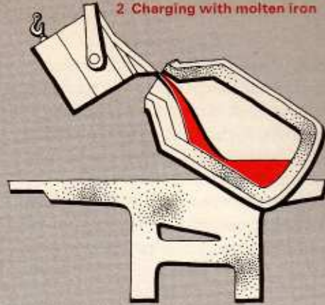
2 Charging with molten iron
