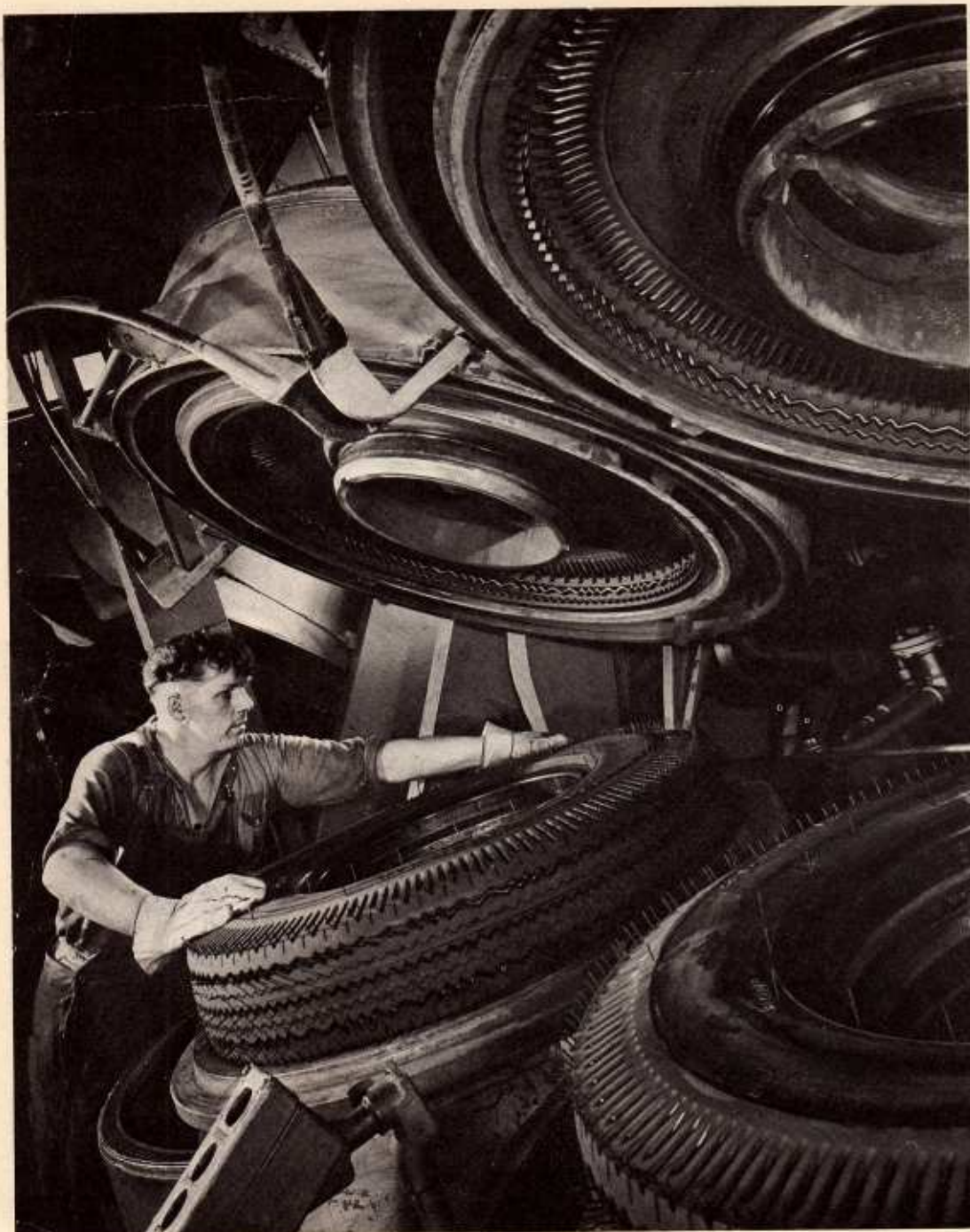
A giant tyre being removed from a vulcanizing press. In the press the rubber is toughened by heating it with sulphur and is moulded into shape. Federation of British Rubber and Allied Manufacturers
