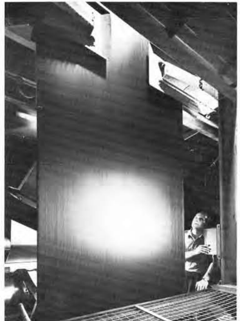
Figure 11 (right) Radioisotope thickness gauge for measuring thickness of tyre cord using 90 Sr. The gauges are at the top corners of the rubber sheet and measure the amount of radiation which passes through the rubber. United Kingdom Atomic Energy Authority.
