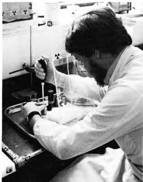
Figure 8 Perspex used to shield a researcher from \beta -radiation. Amersham International, P.L.C.
