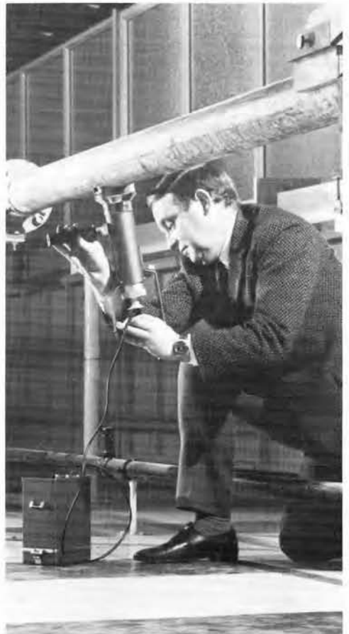
Figure 12 (right) Measuring the thickness of a pipe wall to determine the internal area of the pipe using 137 Cs. Gamma-ray backscattering is the principle used. United Kingdom Atomic Energy Authority.
