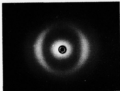
Figure A54 X-ray diffraction pattern for distilled water. Pilkington Brothers P.L.C.
