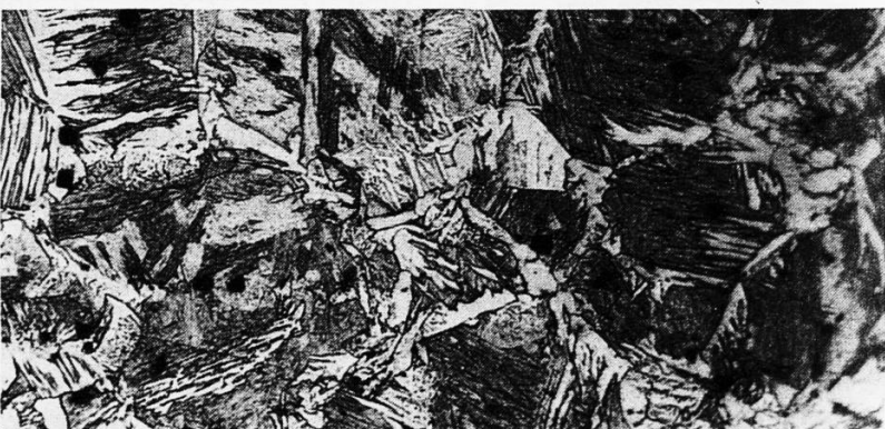
Figure A43 Steel (0.12 % C), quenched (taken at \times 400 ). Note the changes in structure. The dark regions are oxide. Dr A. A. Smith, Faculty of Engineering, King's College, University of London.
