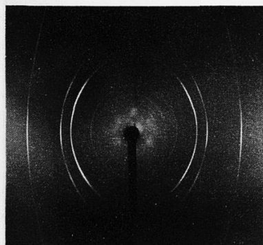
Figure A52 X-ray diffraction pattern for a polycrystalline metal (copper wire). Department of Crystallography, Birkbeck College, University of London.
