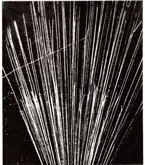
Disintegration of a nitrogen nucleus by an alpha particle. Photograph, Lord Blackett.
